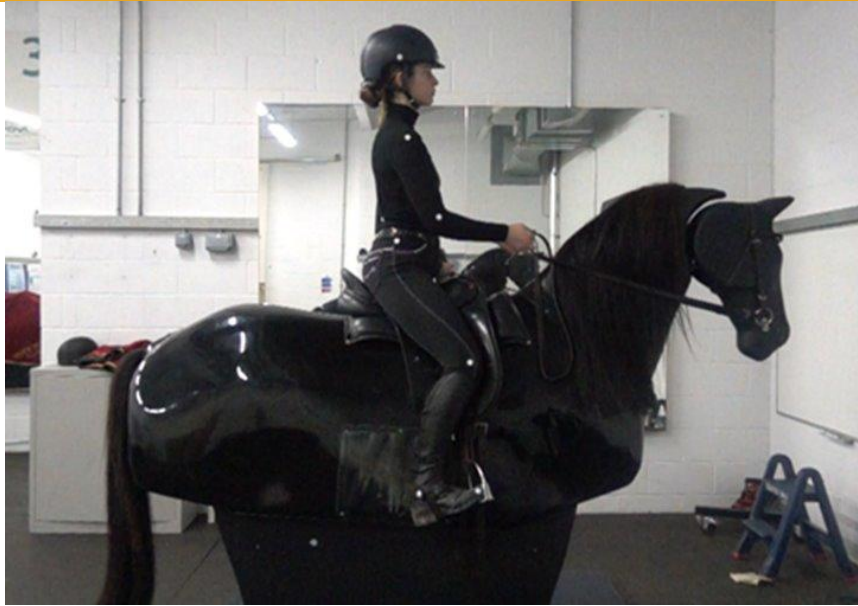
Figure 1: Riding simulators can be used to replace horses within research studies which only need to assess the rider and not the horse.
